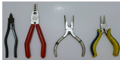
Figure 6. pliers used to band birds. From left to direct, they are exemplified pliers used to open, close and adjust washers and washers shape of hummingbirds. Photo: Anderson Saldanha Bueno.
