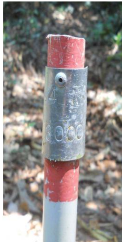
Figure 2. Example of a Figure 3. The picket has an trail marked with pickets. aluminium tag stamped with trail name, and position in meters (3000m in this example). Images: Julio Valley
