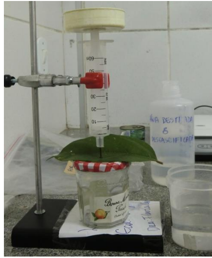
Figure 2. On left, the design of the Chatillon Universal tester to determine force to punch a leaf (figure copied from Arawella et al. 1999) and on the right a simple home-made version of it. A pot is fit over the syringe and gradually filled with water until the weight is enough to perforate the leaf. The leaf must be held in place by hand while pouring gently the water. The marmalade pot bellow the leaf has a hole in the lid, through which the nail attached to the syringe will pass.
