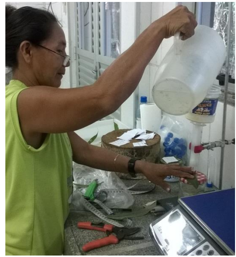
Figure 2. On left, the design of the Chatillon Universal tester to determine force to punch a leaf (figure copied from Arawella et al. 1999) and on the right a simple home-made version of it. A pot is fit over the syringe and gradually filled with water until the weight is enough to perforate the leaf. The leaf must be held in place by hand while pouring gently the water. The marmalade pot bellow the leaf has a hole in the lid, through which the nail attached to the syringe will pass.
