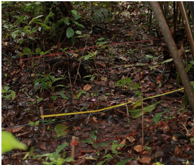
Figure 5. The photo shows (from front to back) the right hand edge of the corridor (red string), the centre line with yellow measuring tape, and the left-hand limit of the sensitive zone (red string).
