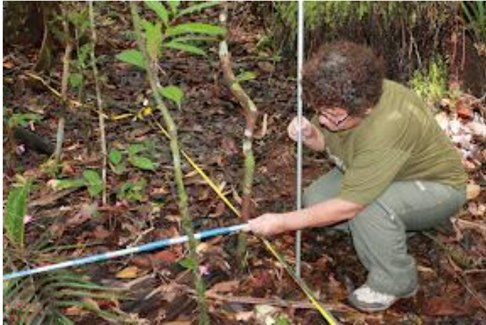
Figure 8. Making a 90° angle.
