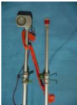
Figure 1: Clinometer and target rod
