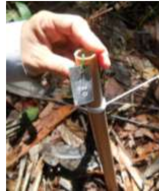
Figure 2: In a 250m survey plot, there will be 52 or more 50cm PVC pickets.
