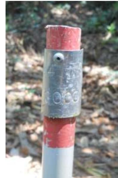
Figure 8- 1m PVC tube with aluminium label showing the location along the trail. This label has been attached using a rivet.
