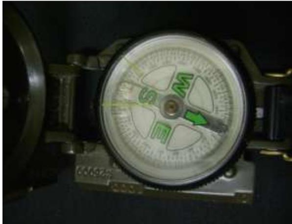
Figure 3 Compass showing magnetic North and the bearing for the trail (marked in yellow).
