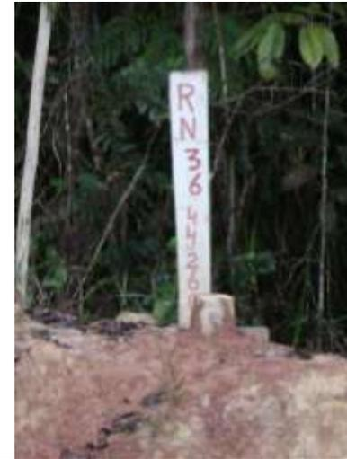
Figure 2. A permanent geo-reference point.
