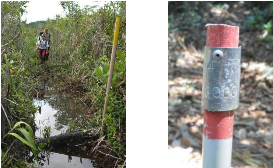
Figure 2. Example of a trail marked with pickets. The picket has a metal plate that shows the track name and the position in meters (3,000 m in the example). Photos: Julio Valley.
