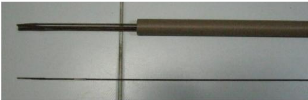
Figure 5. Metal rods for measuring coverage stored in PVC pipe.
