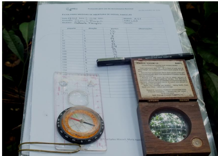
Figure 3: Chart for recording measurements, clipboard, 2B pencil, rubber, plastic bags to protect the clipboard, compass, spherical densiometer metadata and site azimuth data. Picture: Sulamita Marques.
