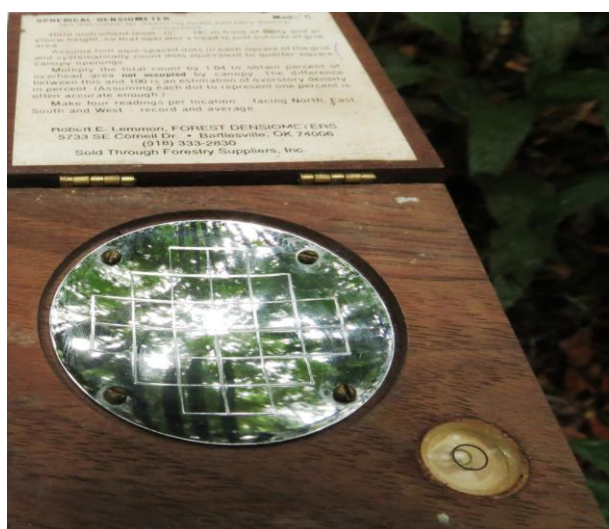
Figure 1: Model C of spherical densiometer, by Robert E. Lemmon, Bartlesville, USA. Picture: Gabriel Masseli.
