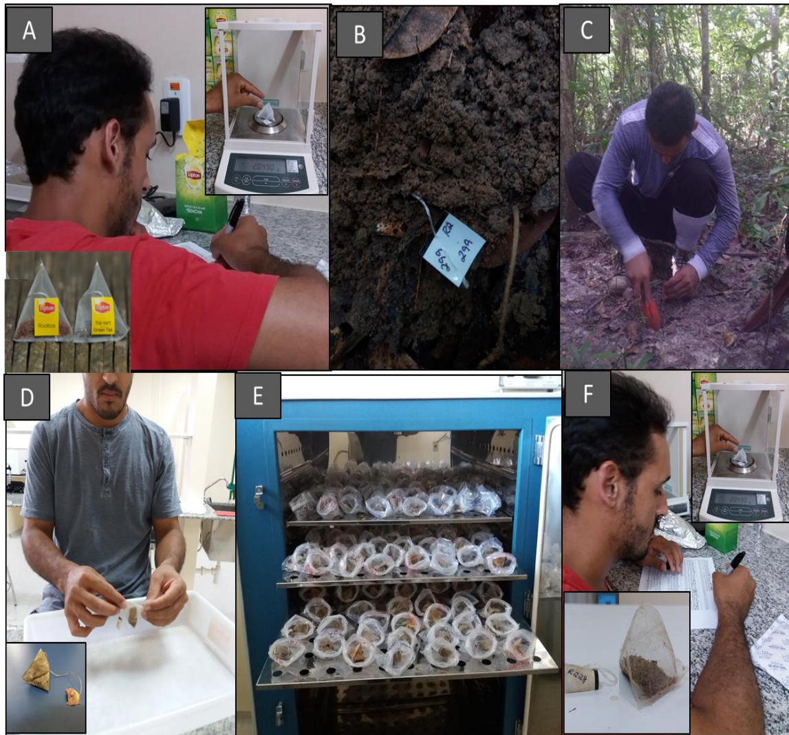
Figure 1 - Methodological procedures for implementation of TBI method: (A) weighing and identification of tea bags, (B) tea bags buried (incubated), (C) withdrawing tea bag, (D) triage of tea bags (physical integrity classification, according to item 9 of the protocol specified below), (E) tea bag drying and (F) tea bag weighing after drying.
